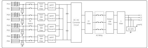
GW50KLV-MT / GW75KW-MT / GW80K-MT PV3 main circuit.
