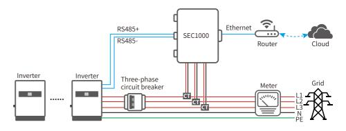
Set related parameters via SolarGo app to enable export power limit control or output power limit control.
