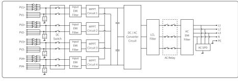
When GW50KN-MT without DC switch, the circuit diagram is as following. For Australia and New Zealand.
