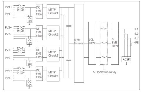
When GW80K-MT is equipped with 3 MPPTs but without DC switch, the circuit diagram is as following. For Australia and New Zealand.
