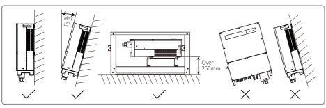
To ensure heat dissipation and convenient disassembly, the minimum clearance around the inverter should not be less than the following values:
