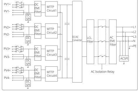
When GW80K-MT is equipped with 4 MPPTs but without DC switch, the circuit diagram is as following. For Australia and New Zealand.
