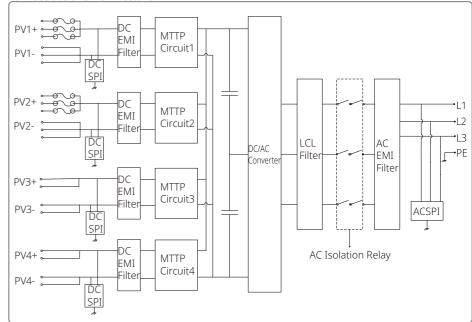
When GW60KN-MT without DC switch, the circuit diagram is as following. For Australia and New Zealand.
