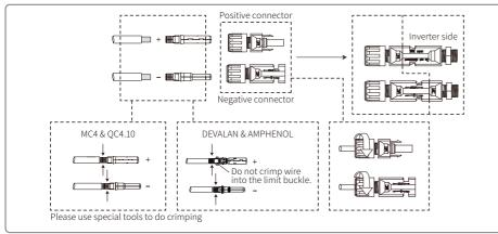
To better dustproof and waterproof the internal inverter, all DC connectors provided in the accessory bag should be connected to the inverter. If only some of the DC connectors are used, the DC connectors without connection should be blocked with a non-conductive insulator.
