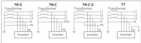
Note: For a TT-grid structure, the RMS voltage between the neutral wire and the earth wire must be less than 20V.
